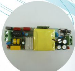
LED driver inside view
